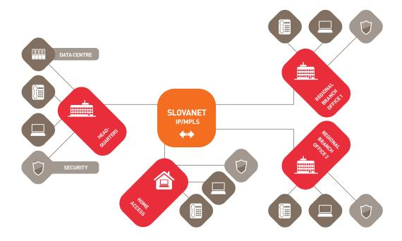
There is not much you need to create a **vpn:LINK**. Each branch office should dispose of at least one computer, which can be connected by an optical, metallic, wireless, ADSL, ISDN or mobile connection. However, the actual technical solution is tailored by us with regard to your needs, whereas we consider both technological requirements and minimum costs.
